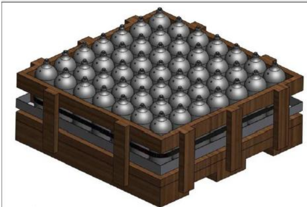
Figure C-3. Example Box Pallet for Shipping 3-Liter Flasks in a 7-Flask by 7-Flask Configuration
